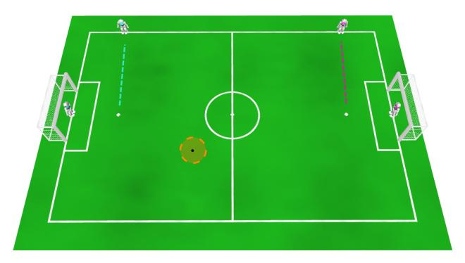
Figure 11: For robots coming back from a standard removal penalty, re-entry points lie in their own half, on the sideline on the side away from the ball.
